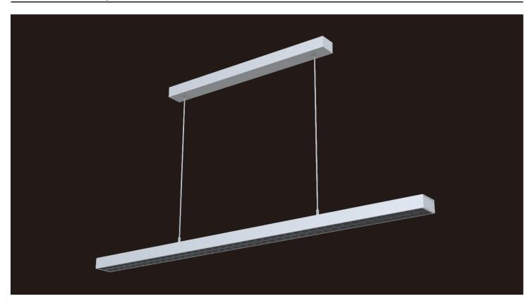
With extremely simple design, excellent craftwork and hidden AC cable, exquisite appearance looks with rich of texture. Lamp is designed with special Direct/Indirect lighting and 110°(Indirect) beam angle. Collocated with micro reflector and anti-glare cover, it can realize 50°(Direct) beam angle and perfect light cutoff. UGR value is as low as 6.
